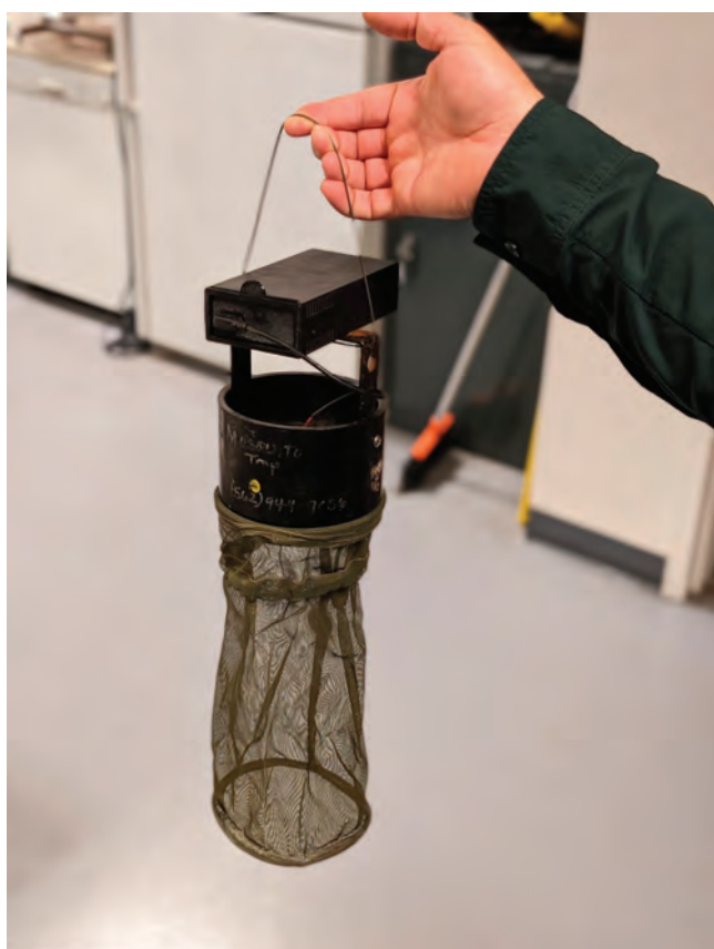
Figure 2. —EVS/CO 2 Trap with an installed 3D printed battery enclosure containing a USB battery pack.
