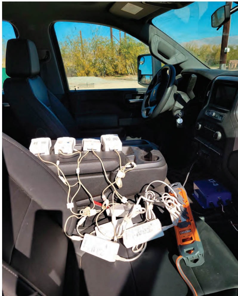
Figure 7.—DJI Phantom 4 Pro UAS battery recharging in the truck cab with air conditioning cooling the batteries.
