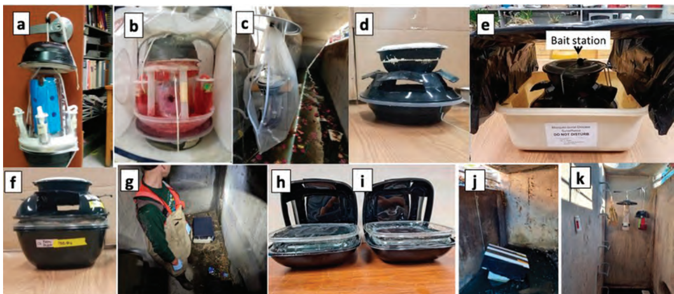
Figure 2. —ATSB station designs. Trap designs shown in chronological order (2018–2022). Hanging ATSB designs used in 2018 (a, b, c) and 2022 (k) included an outer support frame and exposed feeding surface with liquid sugar bait. Floating ATSB designs used in 2019–2022 (d–j) included internal bait reservoirs that mosquitoes accessed through an opening in the trap body. Floating designs were later retrofitted with covers (shown in e, g, j) to prevent damage from water in-flows into the USDS chamber.
