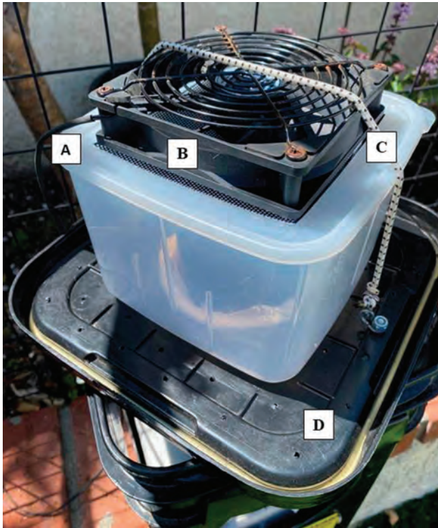
Figure 1. —The Bucket trap showing the collection chamber (A) and fan motor (B) secured in position by an elastic strap (C) fastened across the underside of the bucket lid (D).
