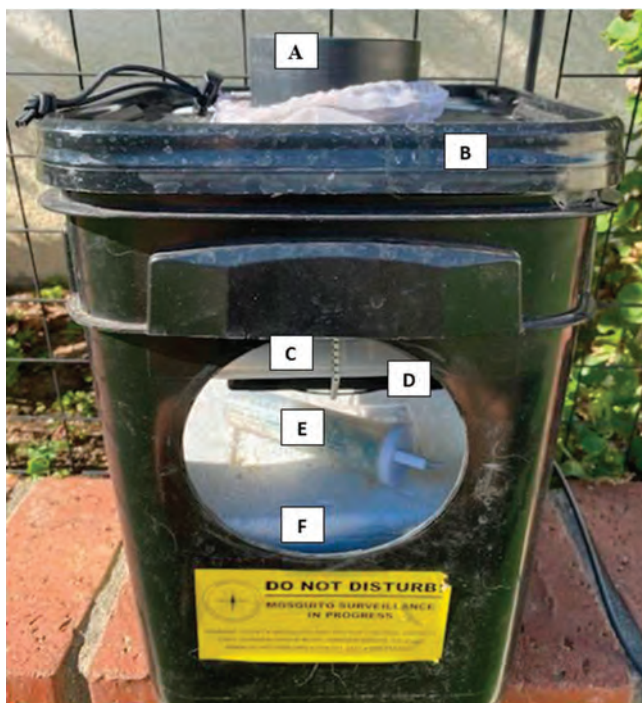
Figure 2. —Configuration of the Bucket trap: A) inlet tube, B) bucket lid seated on bucket, C) collection chamber, D) computer fan motor, E) BG cartridge lure, and F) insulated container.
