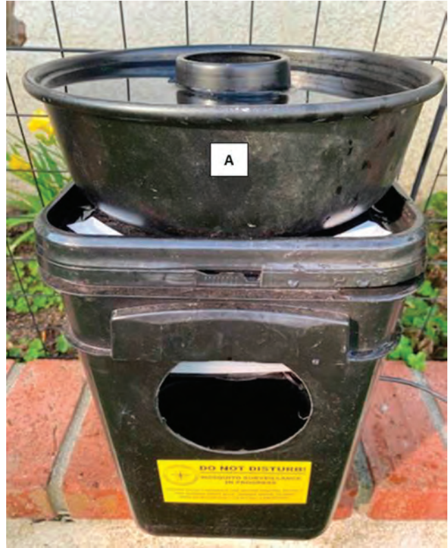
Figure 5. —Bucket trap modified into a gravid trap by placing a Bundt cake pan (A) filled with attractant media for mosquito oviposition over trap inlet tube.
