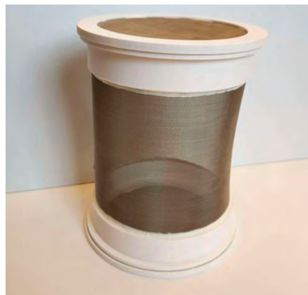
Figure 2.—A fully assembled 3D printed sentinel cage with stainless steel mesh.
