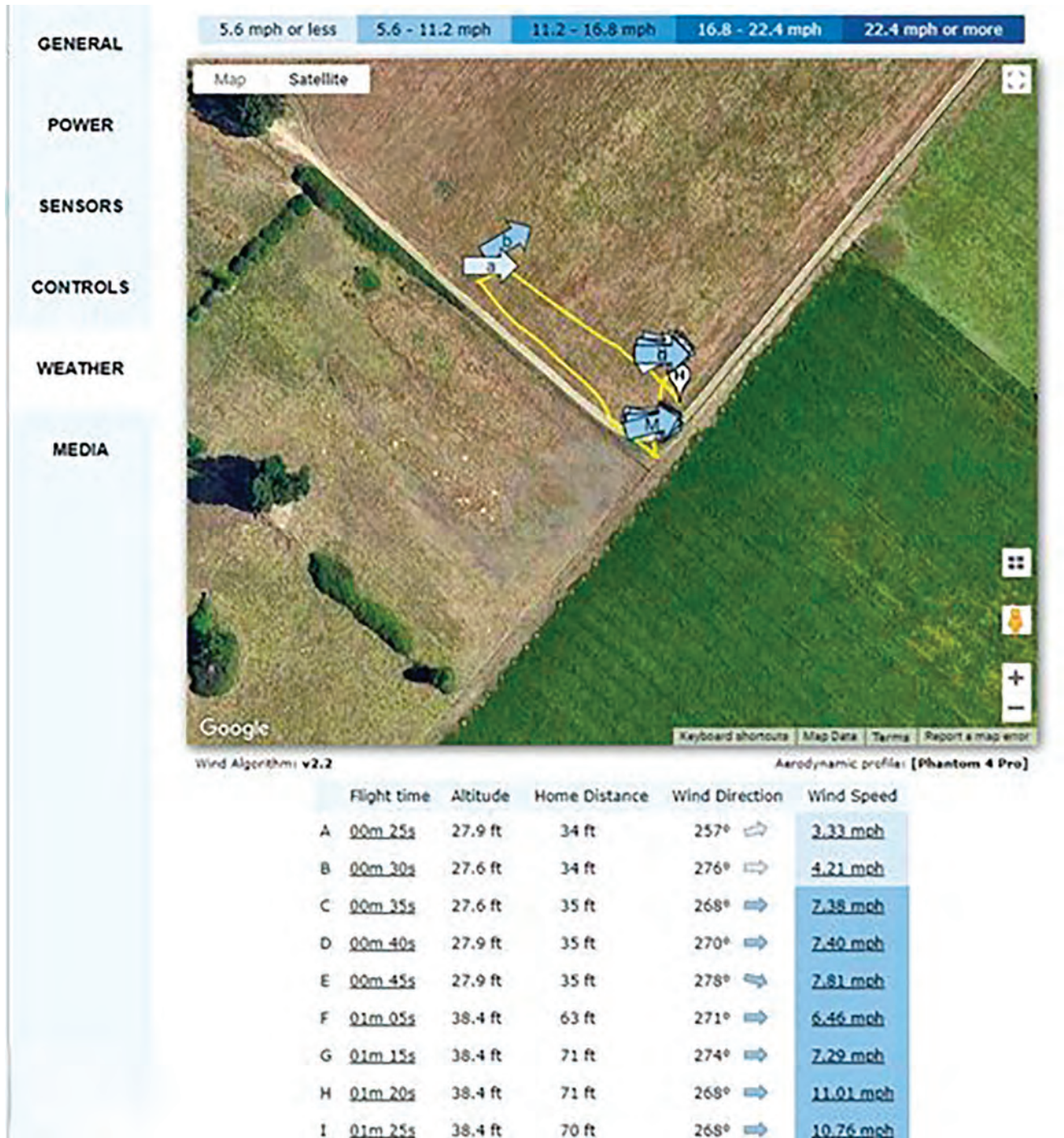
Figure 4.—Map within Airdata.com showing wind speeds and directions at all locations flown during that mission.
