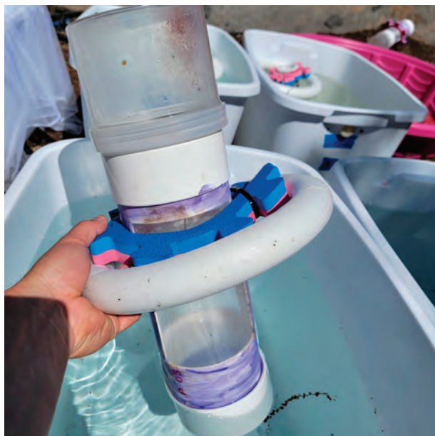
Figure 1.—The previously deployed sentinel cage that was made from irrigation pipe and tulle.
