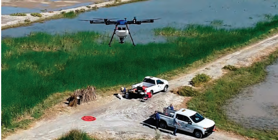
Figure 6.—UAS (Precision Vision 35X) operations at duck clubs near the Salton Sea.
