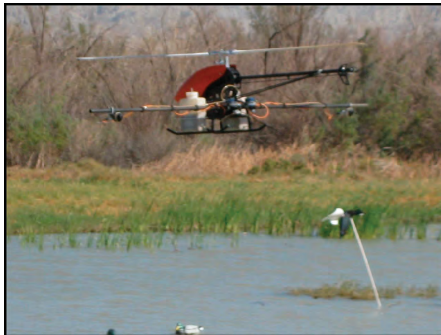
Figure 1.—Leading Edge Aerial Technology remote controlled aircraft equipped with a liquid application system.
