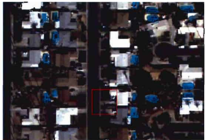
Figure 2. Polygons delineating potential swimming pool locations derived through use of an image segmentation approach.
