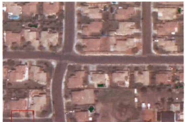
Figure 3. Output of the unsupervised classification scheme, showing candidate neglected pools mapped by the scheme in green, overlaid upon the 2008 image.
