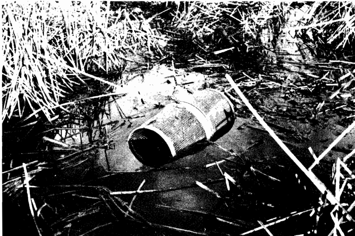
Figure 2. Standard wire minnow trap used to sample fish populations in the units.
